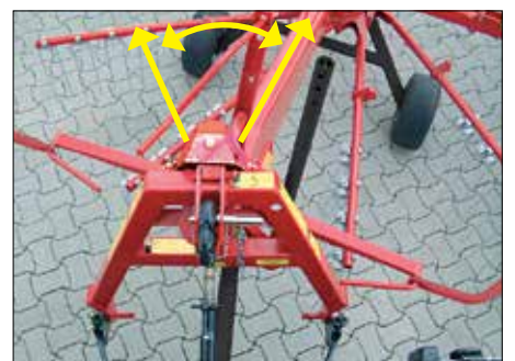
The articulated 3-point headstock ensures that the rake follows the tractor around corners.
