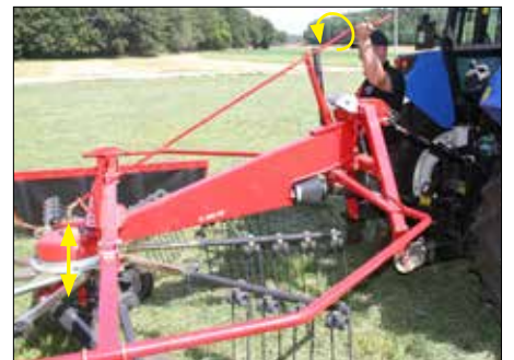
Working height. The working height is easy to adjust with the practical handle above the headstock.
