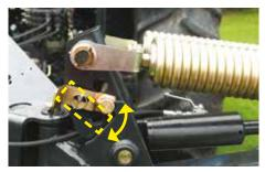
Setting of relief The relief of the machine can be adjusted in several positions so it can be adapted to the local ground conditions.
