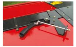
The swath rollers are adjusted in steps by means of a device placed on top of the guard.
