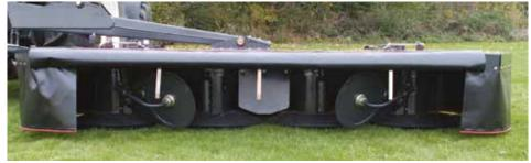
CM 305 can be equipped with 2 adjustable swath rollers which gather the crop to a swath.
