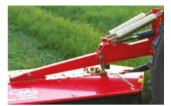
Spring-relieved boom arm CM 305 is suspended in a strong springrelieved boom arm. The two strong springs ensure a smooth operation and a low ground pressure.
