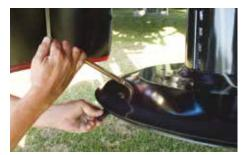
Quick replacement of blades Blades are replaced quickly and easily by means of the supplied ergonomic tool without loosening any bolts or nuts. Press down gently – the blade is released and the new blade can be mounted.
