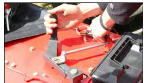
Swath rollers can easily be adjusted from the outside.
