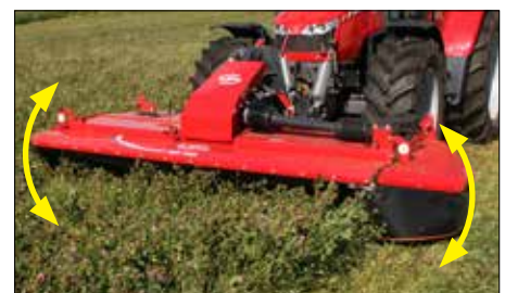
Flexible headstock for perfect ground contour following.
