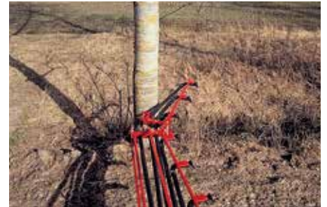
The outer sections of the boom are equipped with a spring-loaded safety break back protection, in order to avoid damage to the boom.
