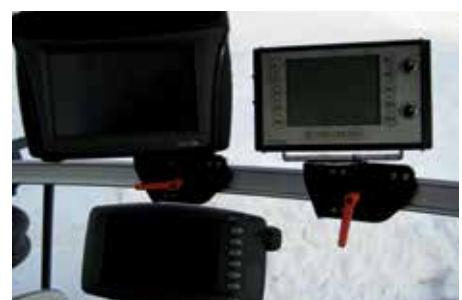
The K-Plus is easily connected to an external GPS or N-Sensor with RS 232 cable.
