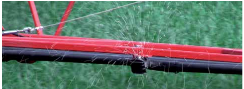
The spreader plates distribute evenly within their working width.
