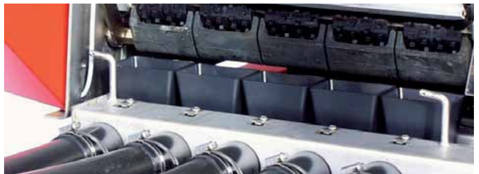
Forced feeding with studded feed rollers mean high precision.
