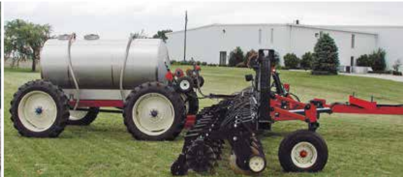
Model F6200 with 1600 Gallon Stainless Steel Tank.
