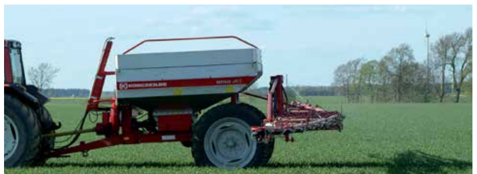
Irrespective of the type of fertiliser being used, the 20 evenly-spaced outlets ensure a negligible effect on the spread pattern by higher wind speeds.
