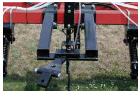
Rear Hitch with extendable tongue.
