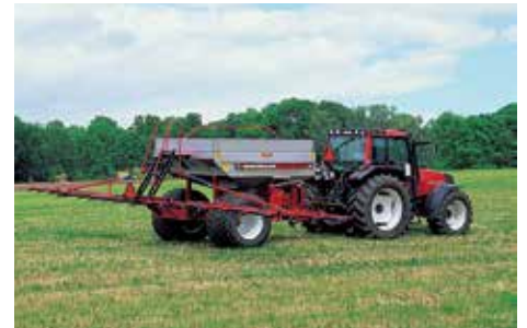
Wing Jet 4012 with 39' working width. 800-26,5 LGP-tires and hopper extension. Loading capacity 6 tons.
