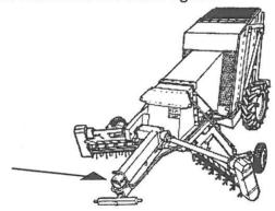
Lifting chains or straps must be of an adequate length in order to avoid abrading or otherwise damaging the Stonebear.
