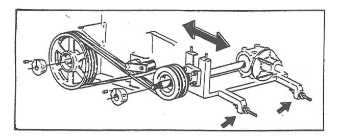
When replacing belts, ensure that they are in the correct position. Belts running to the foremost belt pulley must always run inwards (see illustration). Upon initial application, the new belts will fall into place. This is why driving on new belts must be started carefully and the belt tension must be initially checked at regular hourly intervals.
