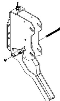
7) Attach the centre spike bar section to the arms by placing the lip of the spike bar angle into one of the 5 notches in the hanger arm and securing the bar in place with the lower spacer, backing plate and U-Bolt.
