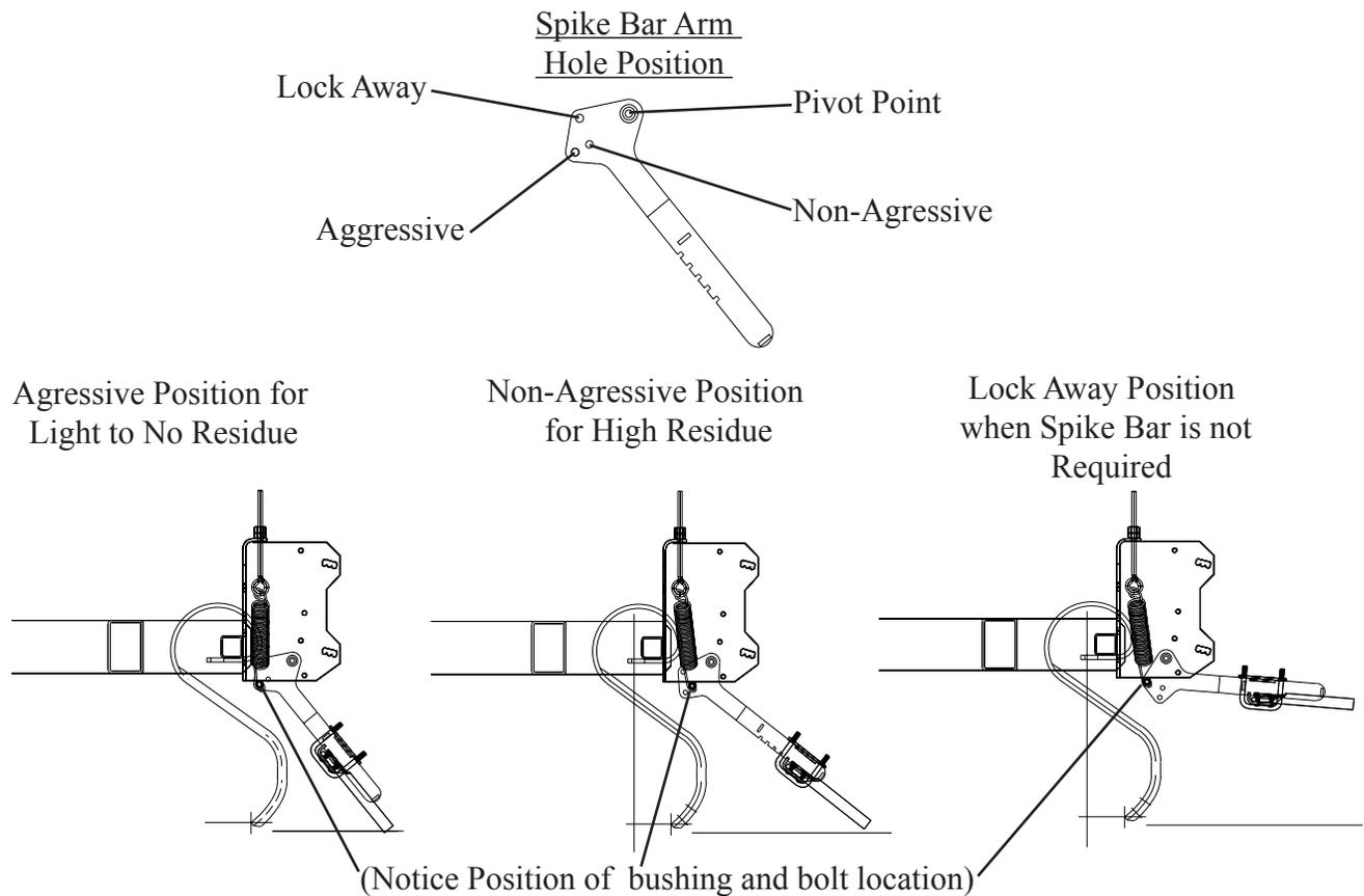
2) The spring pressure can be adjusted to maintain constant spring tension by loosening or tightening the two lock nut on the eye bolt.
