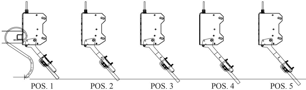
Diagram B shows the effect on the working angle of the arm and how much farther the spring is stretched when the spike bar is lowered.
