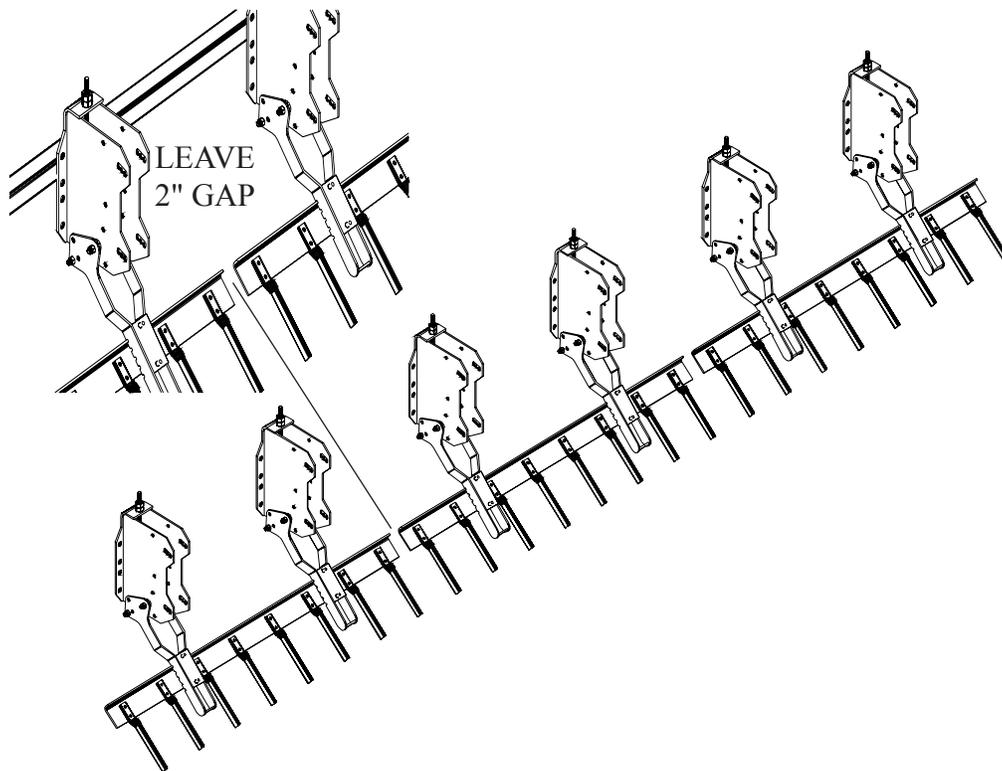
11) When you are satisfied with the spacing of the spike bars and position of the mounting brackets, tighten all nuts and bolts.
