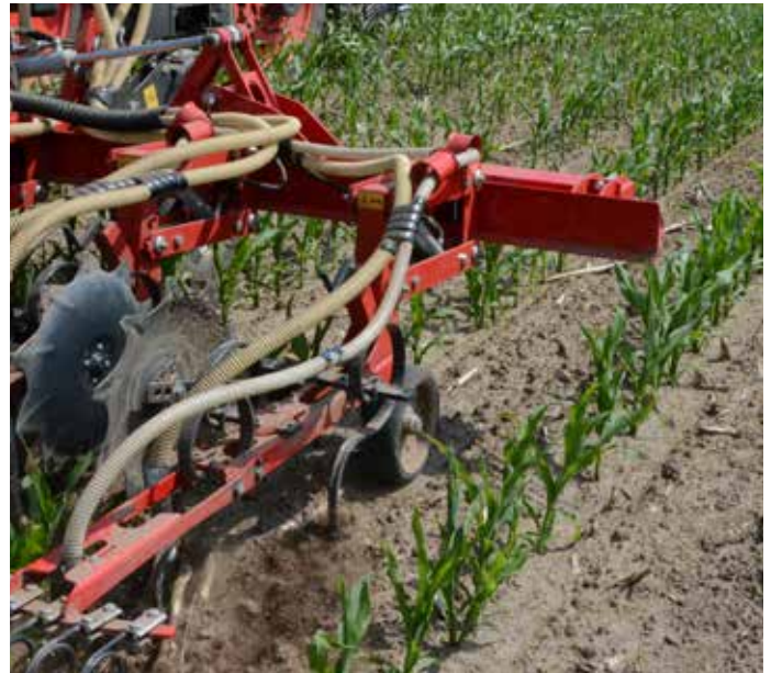
Cleaning sections with genuine Kongskilde tines and shares and rotating plant protection shields for optimum cleaning.
