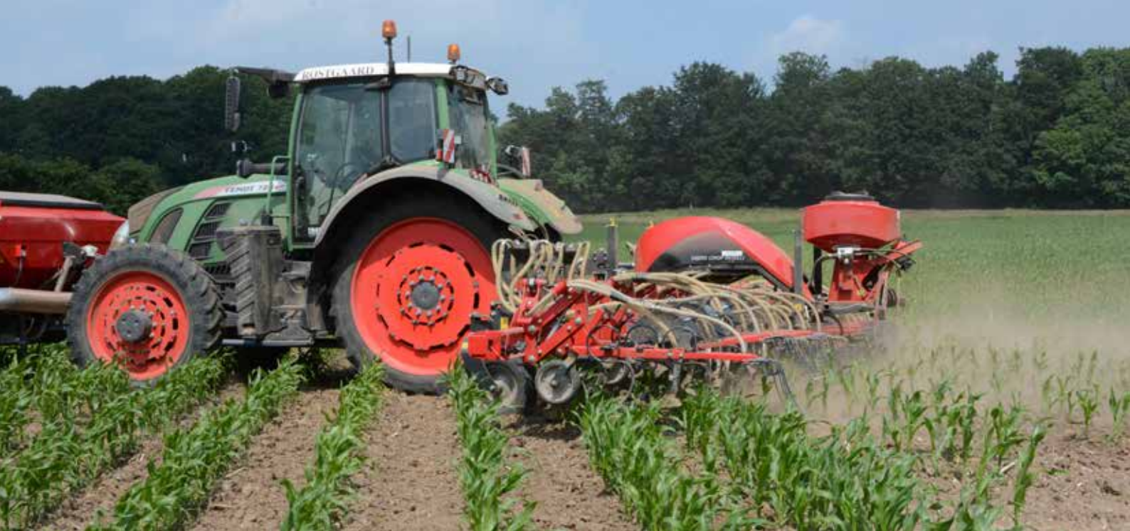
VCO-I with section control - outer section to the left is raised
