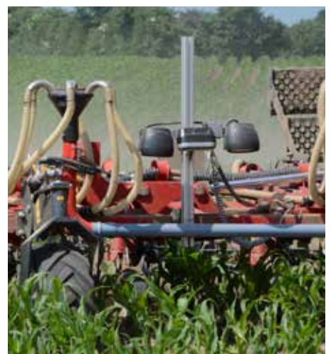
The height and angle of the stereo camera can be adjusted depending on the actual growth stage of the crop.
