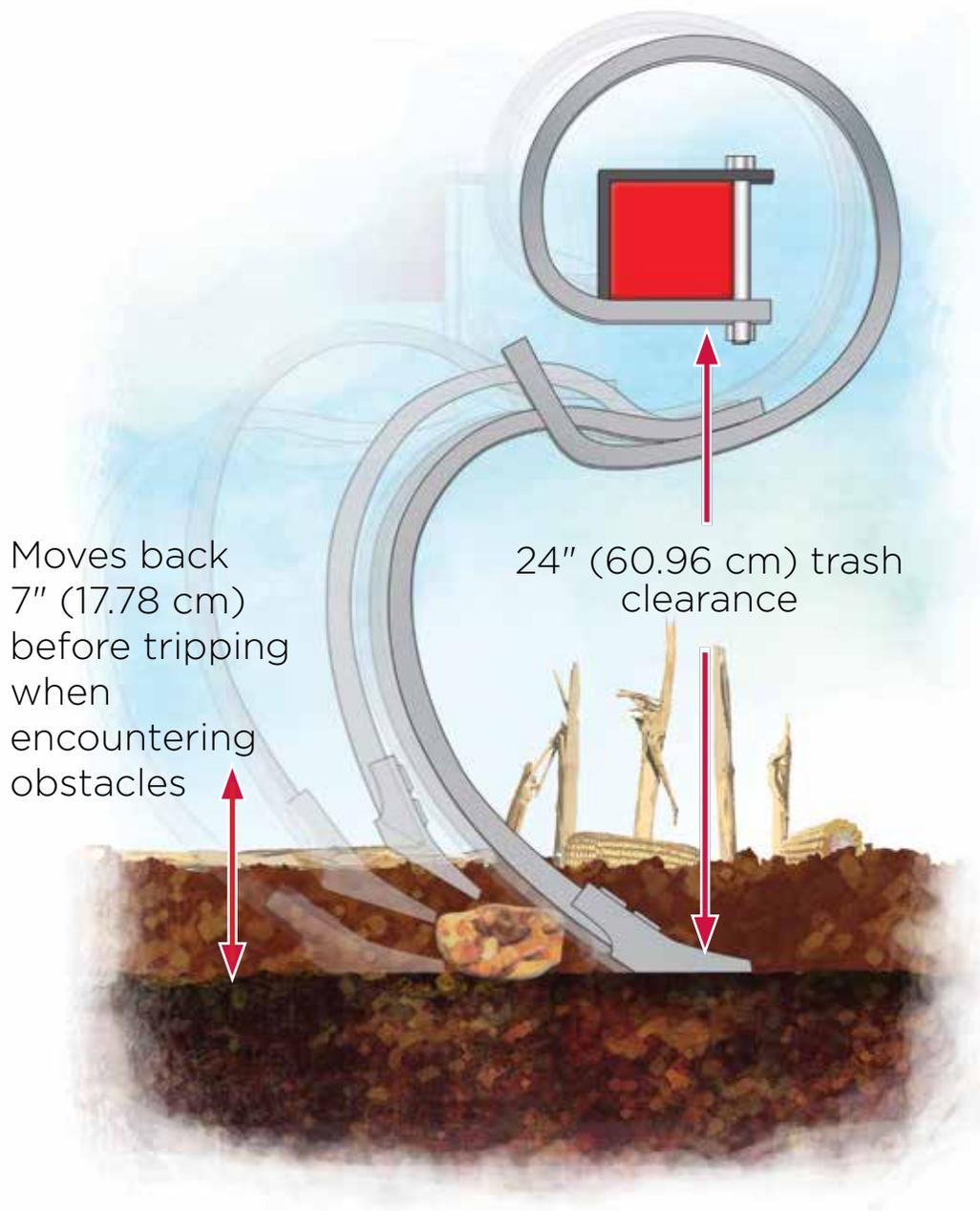
Kongskilde's signature soil bed prep technology starts with our revolutionary S-tine technology. Consisting of three pieces - the coil, the stem and the share - the S-tine breaks through residue like no other shank. The coil's dimension [Standard Duty 0.524" on 4" (10.16 cm) spacing and Heavy Duty 0.624" on 6" (15.24 cm) spacing] ensures the powerful, forward, backward and sideways motion of the tine. Strong enough for first-pass tillage yet vibrant enough to create an ideal seedbed.
