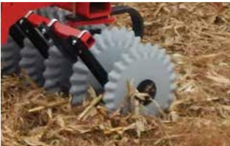
1. Sawtooth SoilRazor VT disk blades cut the trash
