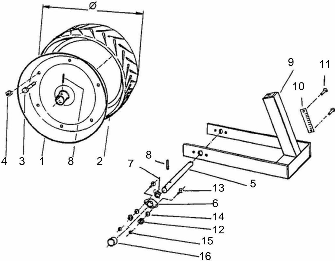
**Spare parts list / Aeromat – Druckrolle Ø 500**
