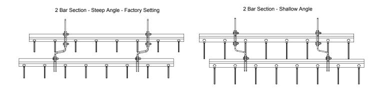
IMPORTANT: If using the shallow angle setting, left and right side harrow arm dimensions in harrow layout manual must be switched: dimension on the right side, used for the left and dimension on the left side used for the right.
