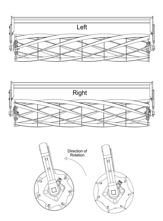
Start assembling the rollers with the front, middle roller in the center section and work out in both directions to the wings. Shift the center roller to the right so that it is 4" right of center and tighten to roller frame. See sample diagram below.
