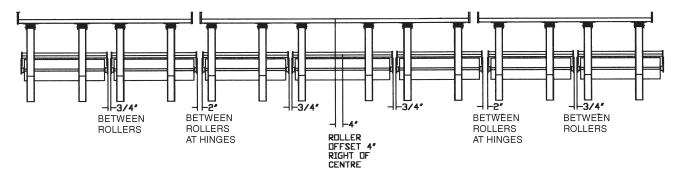
Attach rollers with 3/4" gap between adjacent rollers except where frame hinges leave about a 2" gap as shown above.
