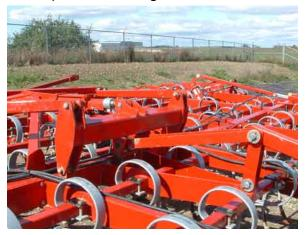
Frequently check the hydraulic system for leaks. Tighten any leaking fittings and carefully inspect the hydraulic lines and replace any worn or damaged hoses. Caution: Hydraulic oil under pressure can be extremely dangerous.
