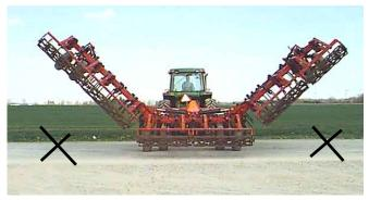
For proper field operation the wing fold cylinders must be fully extended to allow the wings to float. The cyinder rod pin should be centred in the slot in the float position.
