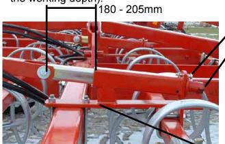
Remove lock pin to make adjustments.
