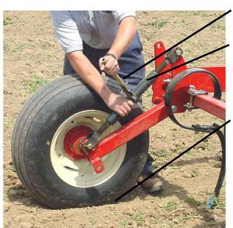
Insert handle and flip lever up or down to make adjustments.
