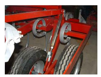
Grease the wheel bearings, hubs and tandem arm pivots weekly, especially before road transtort. Bearing lubrication is recommended more frequently depending on the acreage worked or amounts of road travel involved.
