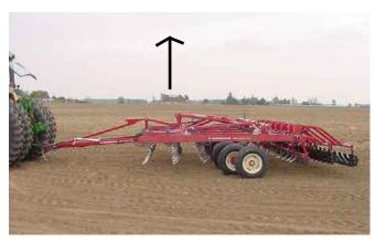
9. Try to avoid making sharp turns when working the soil. Turning with the tines in the ground can cause high stress levels in the cultivator frame and twists the tines, causing premature failure. Sharp turns are especially stressful on the wide wing fold models, as the wing on the inside of the turn may actually try to move backwards in the soil! Lifting the cultivator helps to reduce stress on the cultivator tines and framework.
