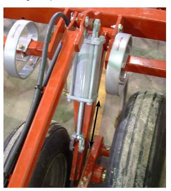
11. The cultivator should never be assembled and placed in the folded position without first charging the hydraulic system, but never assume this has been done! Even on a new machine, leaks can occur from improperly assembled hydraulic components and the folding system could have lost enough oil to allow the wings to free fall to the ground when the unit is unfolded.
