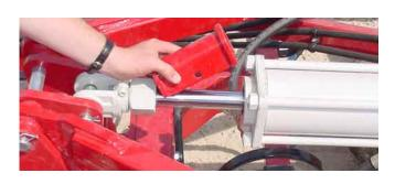
5. Remove the wing lock pins and activate the hydraulics to lower the wings. Check to see that no observers or obstructions are in the path of the wings!
