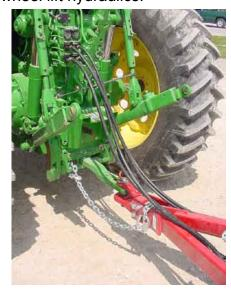
Extend the master wheel lift cylinder and remove transport lock from the centre wheel cylinder rod.
