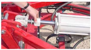
6. The gauge wheels should be adjusted equally to evenly distribute the load across the front of the cultivator and help to maintain fore and aft levelness. The gauge wheels can be adjusted up or down as required by means of the ratchet turnbuckle. Use a tape measure to set each wheel the same.
