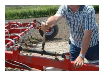
8. Periodically lift the machine completely out of the ground (or when turning at the end of the field). Fully extend the cylinders and hold the remote lever briefly. This rephases the wheel cylinders and keeps the wings at a uniform working depth with the centre section.
