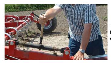
Turn the adjustment turnbuckle to adjust the length of the top link as needed so the machine is running level from front to back.
