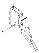
6) Insert a bolt through either of the two holes on the spike leveller arm and, through the bushing holding the spring in place. Fasten the bolt with a locknut.
