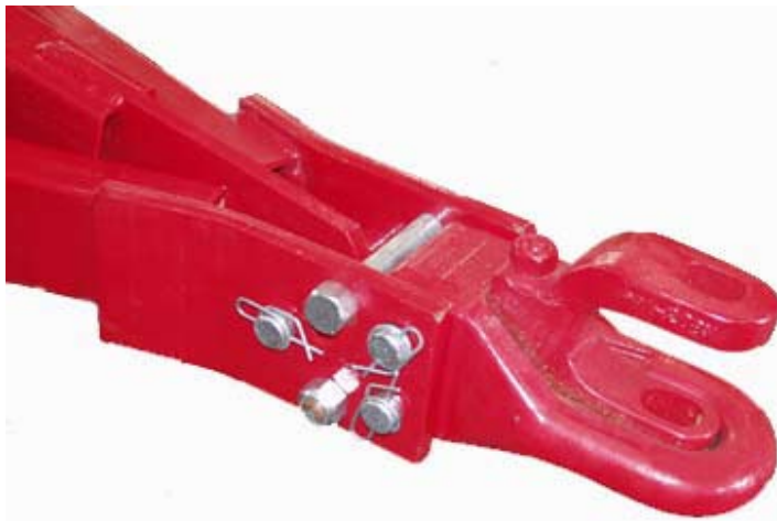
Examples of what the hitch attachment points should look like.
