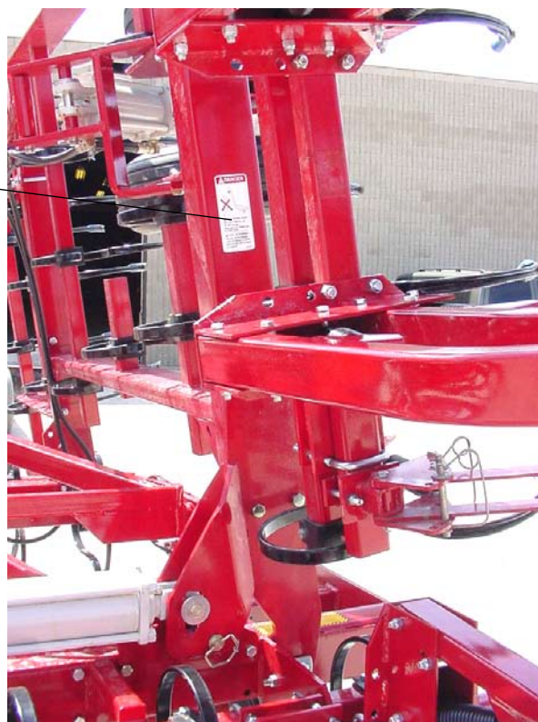
WING SAFETY on rear wing frame tube
