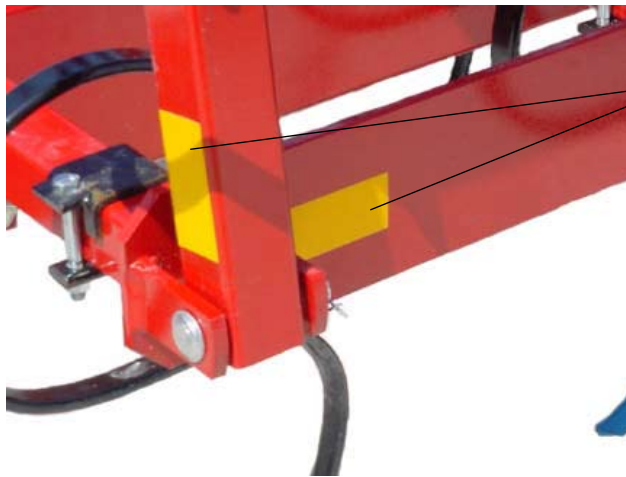
YELLOW REFLECTORS on both front corners and side bars of front frame.
