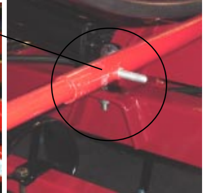
Coarse Adjust: Loosen Set Screw and Slide Tube.
