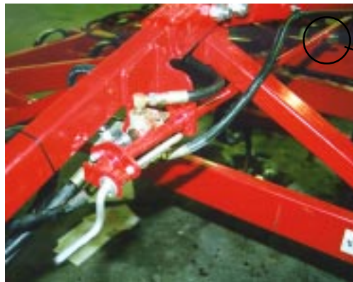
Fine Adjust: Turn Crank Handle to position Striker Bolt.
