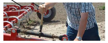
4. After following the previous steps to level the machine, the initial working depth of the tines can be set. This is accomplished by adjusting the mechanical stroke control on the centre section master cylinder out until you are cultivating at the desired depth. The wheel tower sliders and gauge wheels can then be fine tuned so that the wings work level and at the same depth as the centre section.
