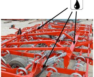
2. Grease the wheel bearings, hubs and tandem arm pivots weekly, especially before road transtort. Bearing lubrication is recommended more frequently depending on the acreage worked or amounts of road travel involved. 3. Inspect the wheel arm pivot points and linkages regularly for signs of excessive wear.
