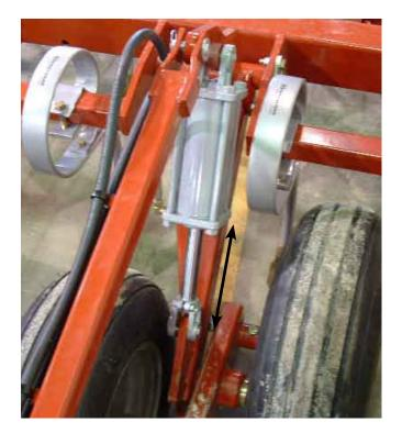
11. The cultivator should never be assembled and placed in the folded position without first charging the hydraulic system, but never assume this has been done! Even on a new machine, leaks can occur from improperly assembled hydraulic components and the folding system could have lost enough oil to allow the wings to free fall to the ground when the unit is unfolded.
