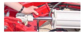
5. Remove the wing lock pins and activate the hydraulics to lower the wings. Check to see that no observers or obstructions are in the path of the wings!
