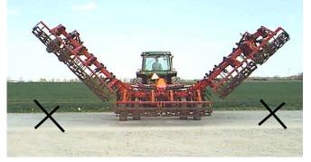
6. For proper field operation the wing fold cylinders must be fully extended to allow the wings to float. The cyinder rod pin should be centred in the slot in the float position.
