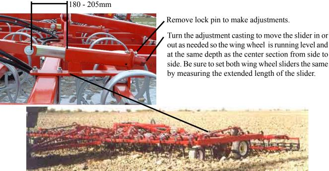
Note how the cultivator wings in this photograph are running higher than the center section. Therefore the wheel adjuster should be lengthened to lower the wing wheels and make the wings level with the centre frame.
