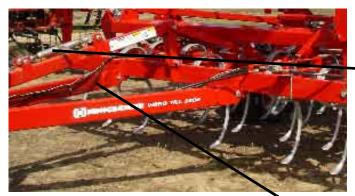
Turn the Turnbuckle to lenghten or shorten the to link as needed so the machine is running level from front to back.
