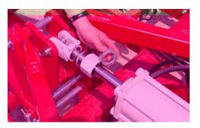
6. The gauge wheels should be adjusted equally to evenly distribute the load across the front of the cultivator and help to maintain fore and aft levelness. The gauge wheels can be adjusted up or down as required by means of the ratchet turnbuckle. Use a tape measure to set each wheel the same.
