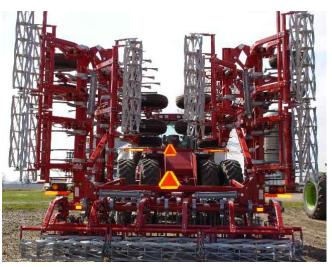
IMPORTANT NOTE: This unit has a narrow transport width and a high centre of gravity which may pose a tipping hazard when folded for transport.
