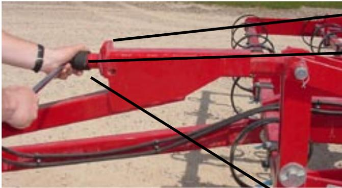
Remove lock pin to make adjustments.
