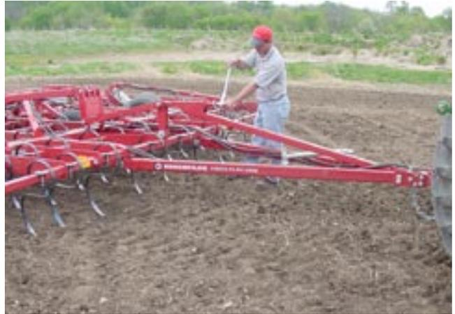
8. Periodically lift the machine completely out of the ground (or when turning at the end of the field). Fully extend the cylinders and hold the remote lever briefly. This rephases the wheel cylinders and keeps the wings at a uniform working depth with the centre section.
