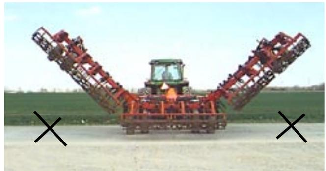
6. For proper field operation the wing fold cylinders must be fully extended to allow the wings to float. The cylinder rod pin should be centred in the slot in the float position.
