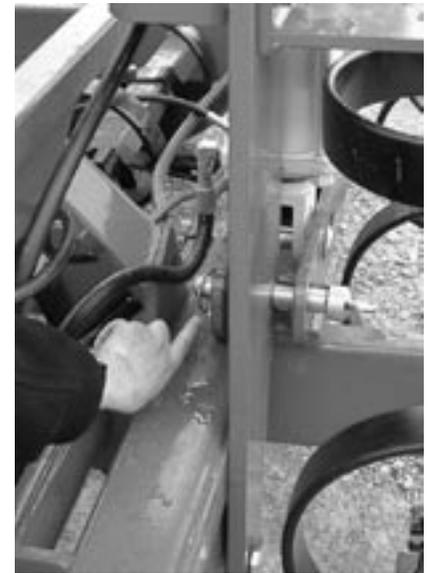
2. When parking the unit in the transport position, ensure that the unit is stable by blocking the wheels to prevent the unit from rolling when disconnected from the tractor.
