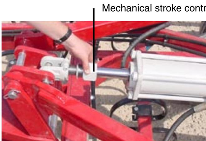
Mechanical stroke control
