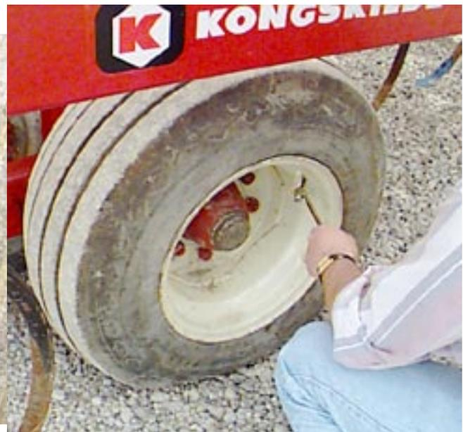
5. Check all nuts and bolts, especially the tine clamp bolts, after the first few hours of operation and secure if loose. Inspect the shares daily and replace worn ones.
