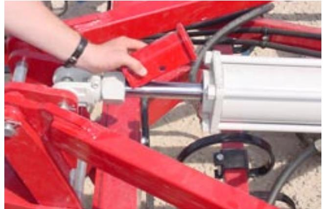
5. Remove the wing lock pins and activate the hydraulics to lower the wings. Check to see that no observers or obstructions are in the path of the wings!
