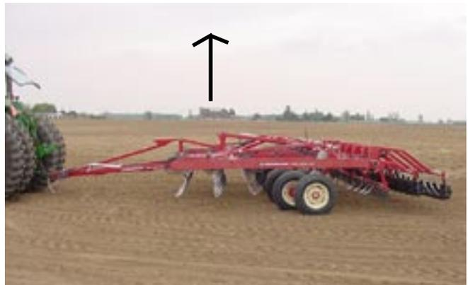
9. Try to avoid making sharp turns when working the soil. Turning with the tines in the ground can cause high stress levels in the cultivator frame and twists the tines, causing premature failure. Sharp turns are especially stressful on the wide wing fold models, as the wing on the inside of the turn may actually try to move backwards in the soil! Lifting the cultivator helps to reduce stress on the cultivator tines and framework.
