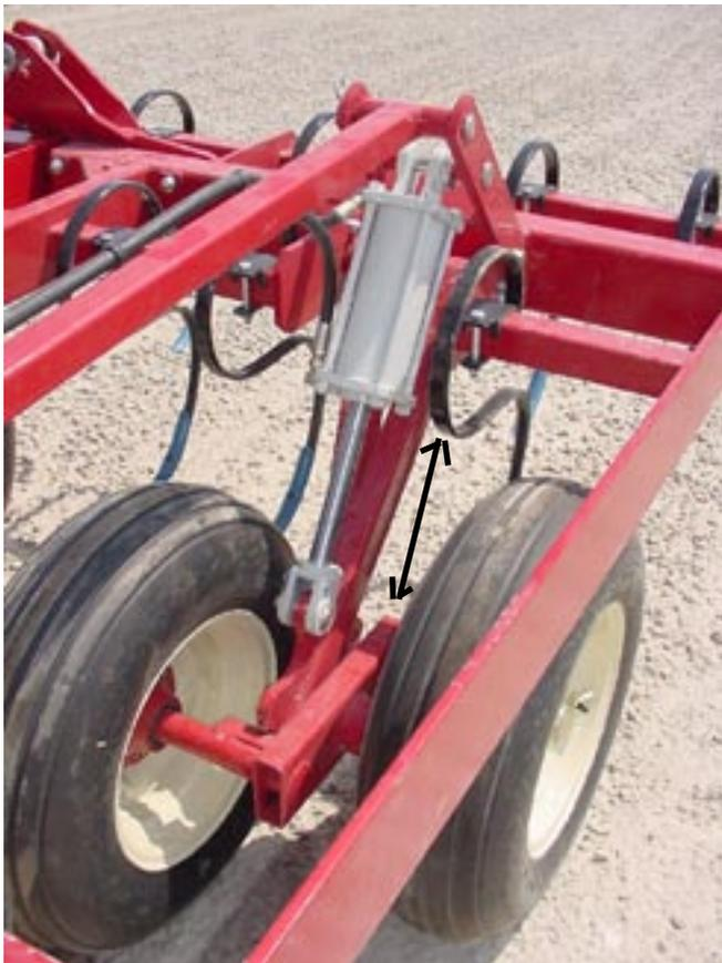
11. The cultivator should never be assembled and placed in the folded position without first charging the hydraulic system, but never assume this has been done! Even on a new machine, leaks can occur from improperly assembled hydraulic components and the folding system could have lost enough oil to allow the wings to free fall to the ground when the unit is unfolded.
