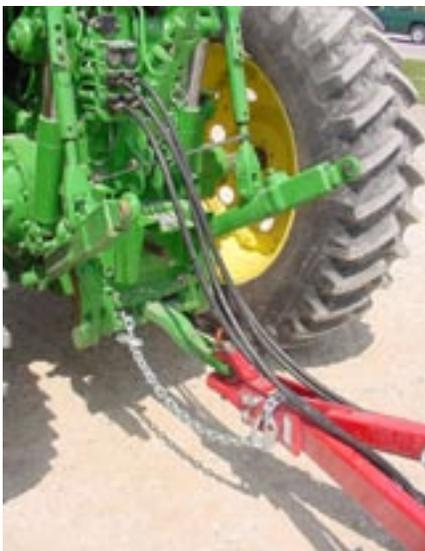
4. Extend the master wheel lift cylinder and remove transport lock from the centre wheel cylinder rod.
