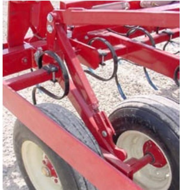
2. Grease the wheel bearings, hubs and tandem arm pivots weekly, especially before road transport. Bearing lubrication is recommended more frequently depending on the acreage worked or amounts of road travel
