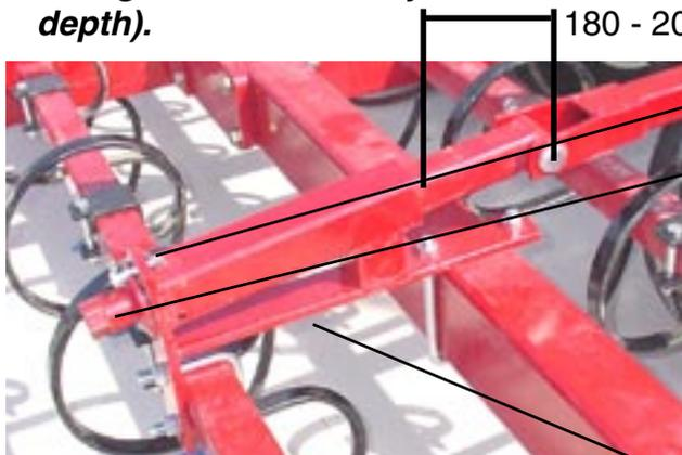
Remove lock pin to make adjustments.
