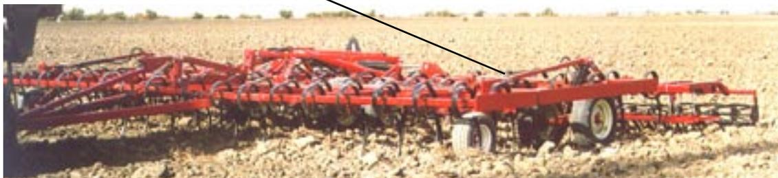
Note how the cultivator wings in this photograph are running higher than the center section. Therefore the wheel adjuster should be lengthened to lower the wing wheels and make the wings level with the centre frame.
