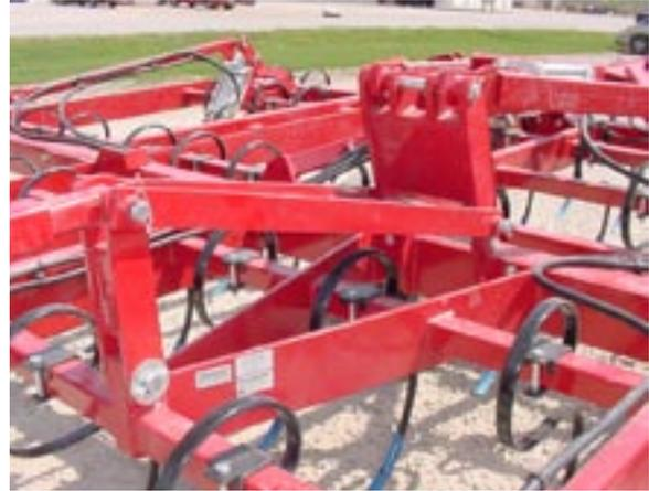
8. Frequently check the hydraulic system for leaks. Tighten any leaking fittings and carefully inspect the hydraulic lines and replace any worn or damaged hoses. **Caution:** Hydraulic oil under pressure can be extremely dangerous.
