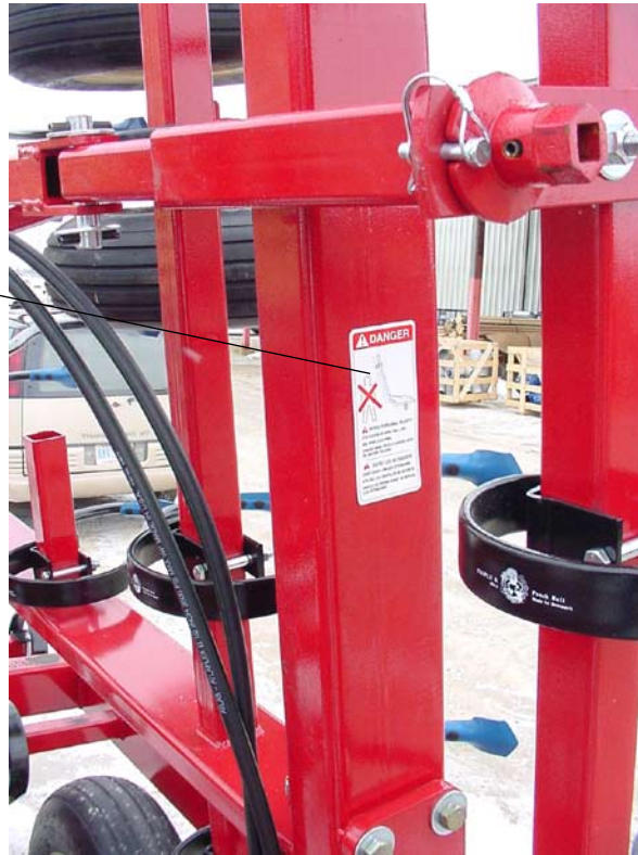
WING SAFETY on front wing frame tube
