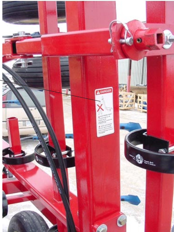
WING SAFETY on front wing frame tube
