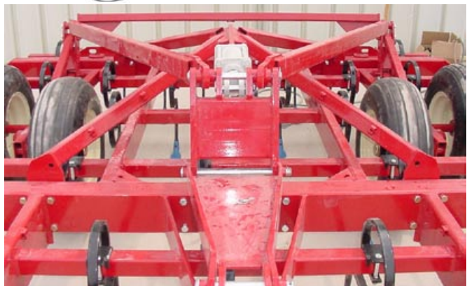
Overview of completed 10' (3m) self levelling linkage system.
