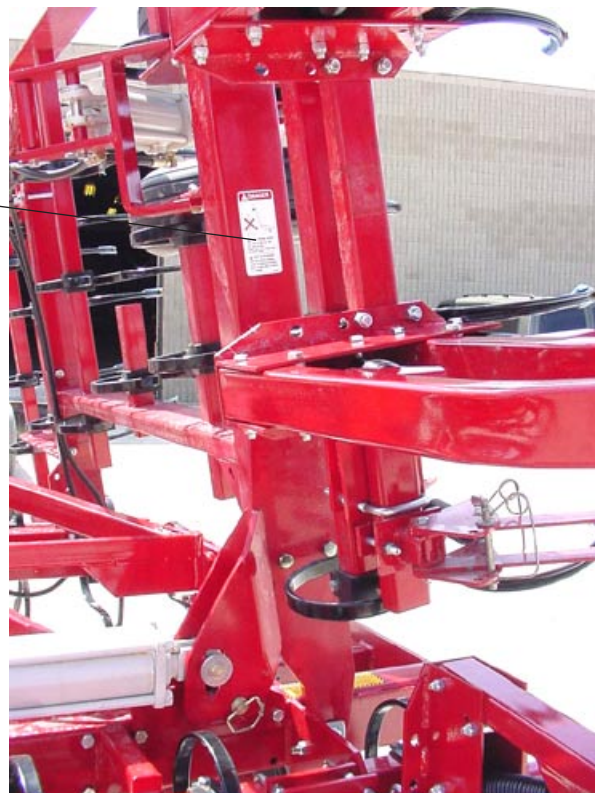
WING SAFETY on rear wing frame tube
