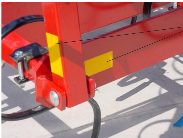
YELLOW REFLECTORS on both front corners and side bars of front frame.
