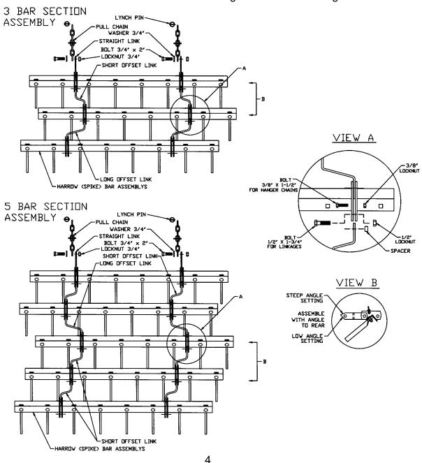
4. <u>Note:</u> On some cultivator models you will need to mount a special extension to the ends of the spike bars. Mark the locations for the bolt holes, or clamp the extensions to the spike bar and use them as a guide for drilling. Secure with bolts and locknuts supplied. See detail below.
