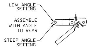
Pre-Assembled Harrows may be changed in the field by disassembling the offset brackets, and then flipping them over and reassembling opposite to the original offset. This modification to the linkages is time consuming but will allow you to change the harrow working angle setting should you find the original set up is not providing the desired results.
