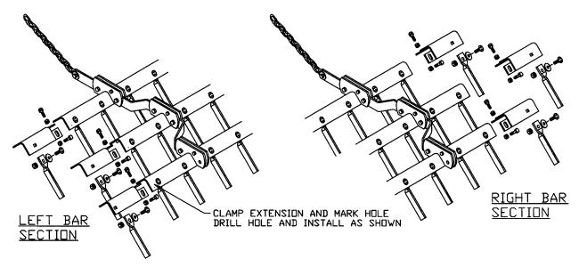
5. Mount the carrier arms to the rear accessory tube of the cultivator centre section with the U-bolts, washers and locknuts provided. Position the arms directly above the chain brackets on the drag harrow assemblies according to the diagram below.
