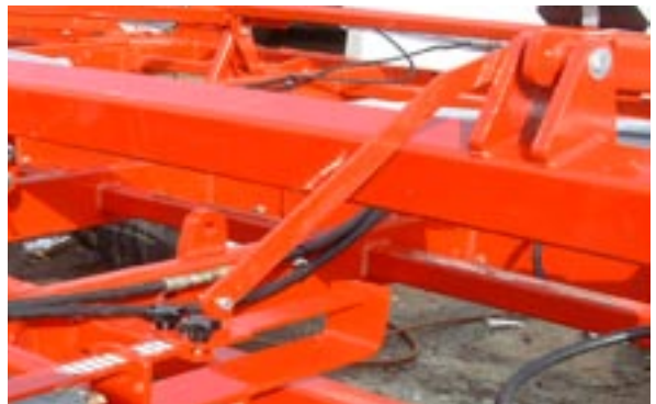
Overview of the completed self-levelling linkage system.
