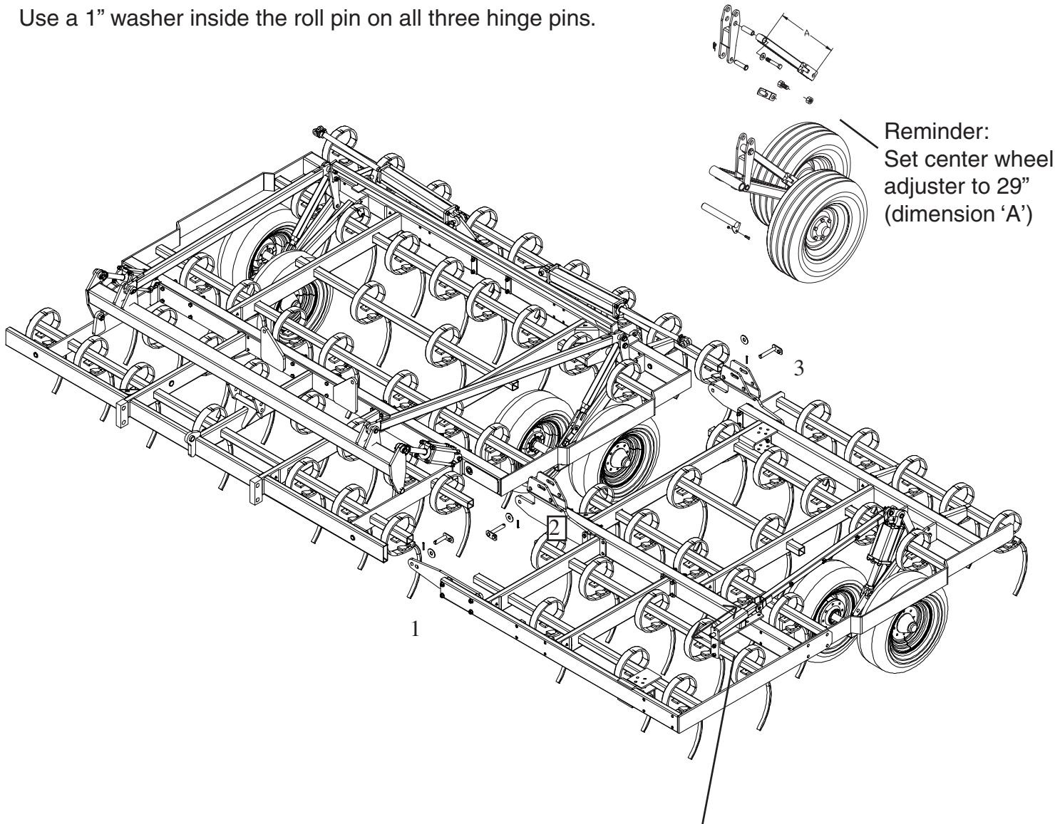
Make sure the wing adjustment slider is cranked out to 7 - 8" **before** raising the machine with the cylinder. If not, a tine could hook itself over the wheel axle, requiring you to remove the tine to unhook it.
