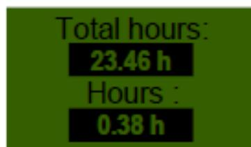
Operating hours counter = running time of sowing shaft.
