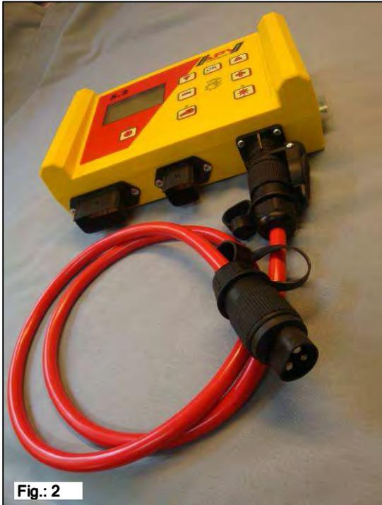
You can connect the cable, provided as part of the standard delivery, directly to the 3-pin standard socket in the tractor cab. Connect the other end to the control module.
