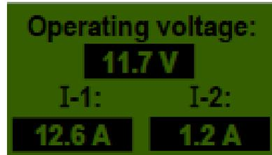
**I-1:** Displays the fan motor's power consumption in amperes.
