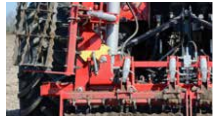
Hydraulic or mechanical wing lock system for safe road transport and convenient operation from the tractor cab.
