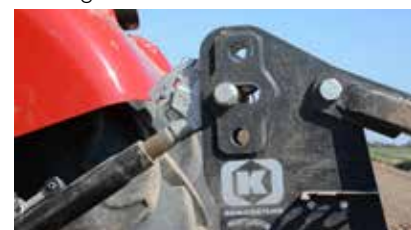
Slotted hole in the topmast helps the cultivator to follow the soil surface in hilly conditions.
