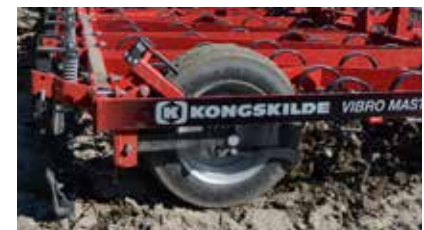
4 large rubber wheels running in front of the tines on firm soil for even depth control.
