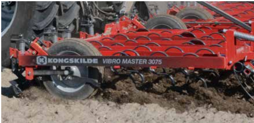
Hydraulic or mechanical wing lock system for safe road transport and convenient operation from the tractor cab.
