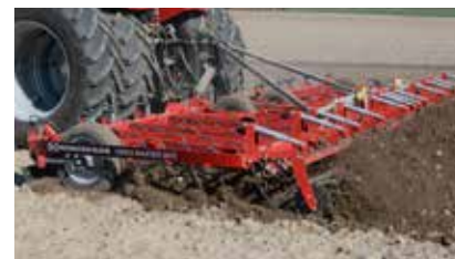
5 rows of tines in a symmetrical pattern ensuring a blockage-free passage of soil and residues.
