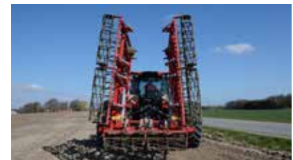
Vertical folding to maximum 3,0 m transport width.
