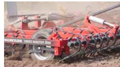
Hydraulic flexboard for crushing and leveling of the soil surface before entering the cultivation zone. Wearing parts can be adjusted.
