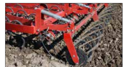
Rear harrow attachment system gives varying roller pressure and attack angle options.
