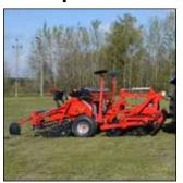
Hydraulic drill linkage - working position.
