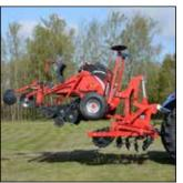
Hydraulic drill linkage - transport position.
