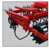
Depth adjustment with pin/hole system.
