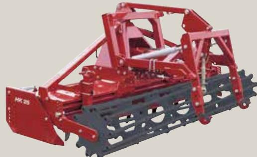
HK 25 with crumble roller and hydraulic Hitch (optional).
