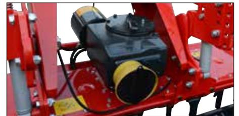
3-speed leverchange gearbox with rear PTO.
