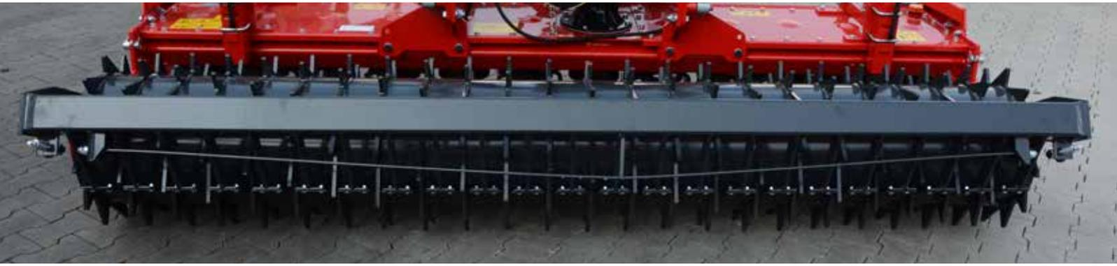
Ultimate versatility is essential and the wide selection of rear rollers enables the Howard Power Harrows to be perfectly suited to different soils and conditions. The right choice of roller also enables effective cultivation and drilling when the Howard Power Harrow is used in combination with a seed drill.
