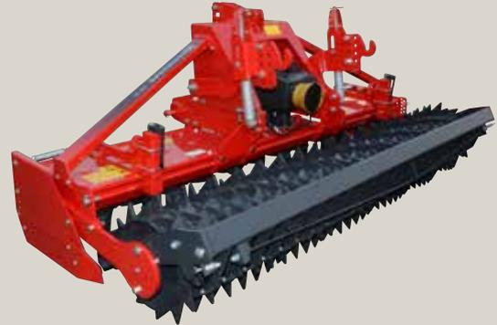
The HK 31 Power Harrow is a Power Harrow for medium and big size farms to work behind tractors up to 125 kW (170HP). A machine which is based on Howard's long experience on PTO driven soil working machines to meet the latest demands of farmers and contractors.
