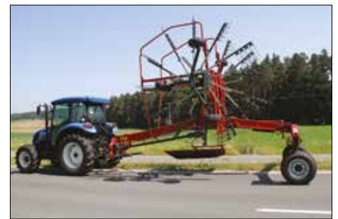
R+ 820 in transport position. The transport height is under 4 m.
