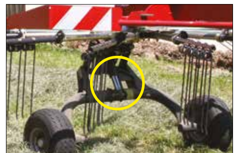
R+ 1410 SB with automatic steering for sharp bends. With the auto-steering the overlap between the rotors are obtained
