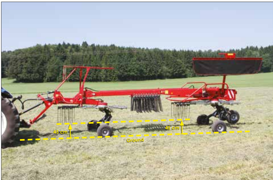
R+ 1410 S - a side delivery rake with Multi Link frame
