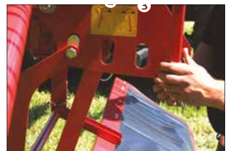
All centre swath rakes have variable working width. You can remove the canvas and use the hole to get an even smaller working width. This could be relevant when working in alfalfa.
