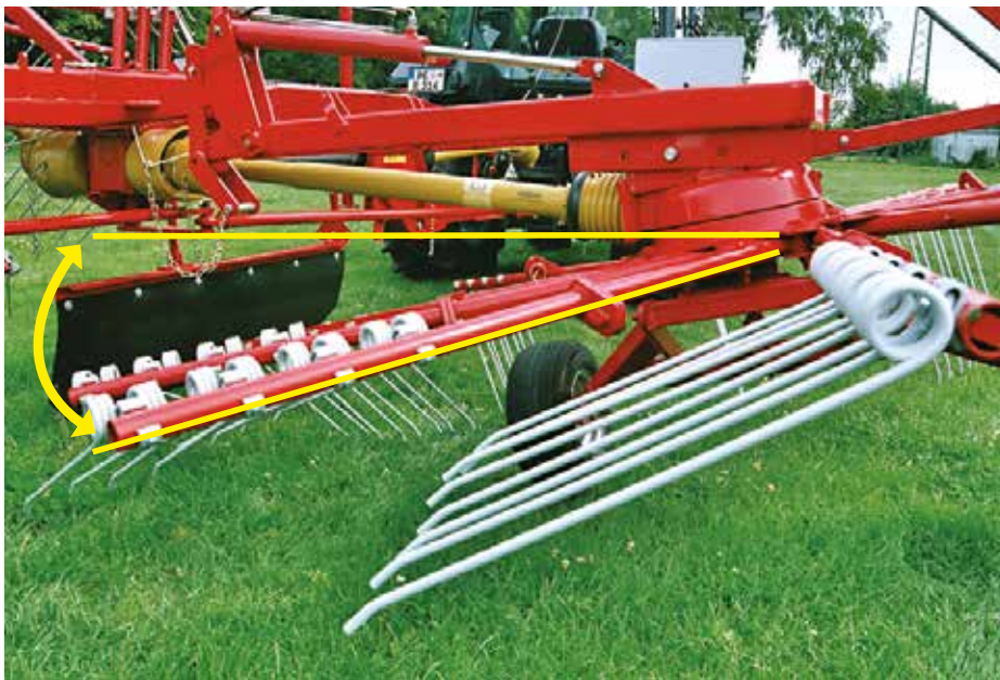
Rotor is not cardanic suspended. Swinging rotor only
