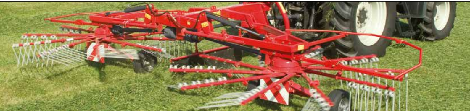
R655 DS - 3-point mounted centre swath rake.
