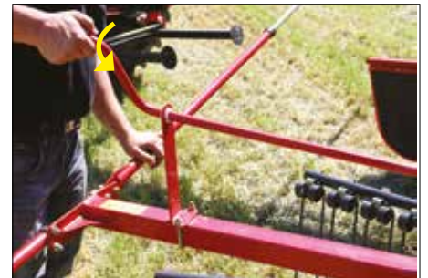
Adjustment of working depth. Simply carried out by manual remote handle – infinite adjustment.
