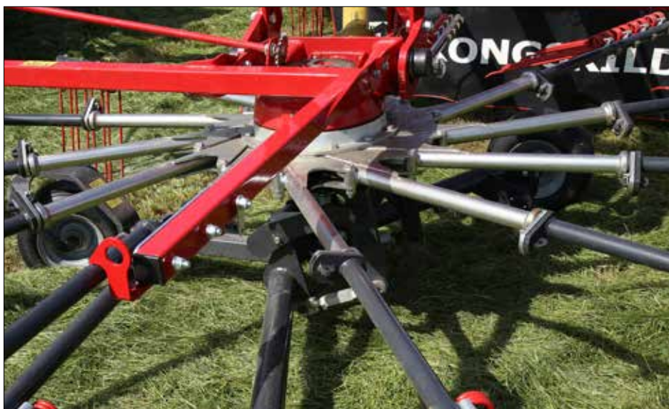
Rotor construction with exchangeable arms
