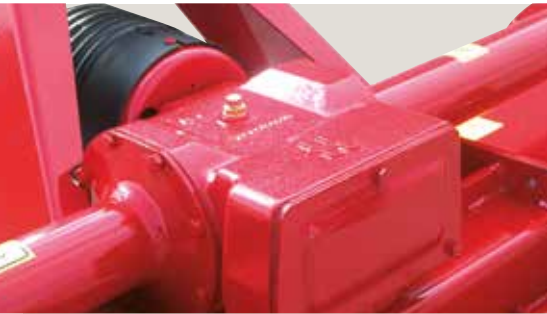
Standard Selectatilt gearbox. The speed is adjusted to the desired finish.
