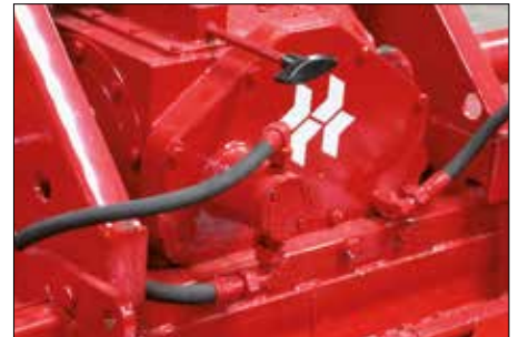
Rotavator 700S-D gearbox. Lever change gearbox and oil cooling system.
