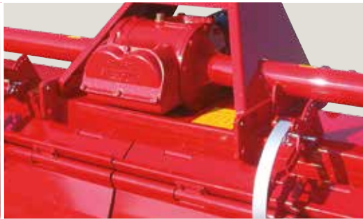
Reinforced Selectatilt gearbox for 280 and 305 working width. It can be mounted to tractors up to 125 HP.
