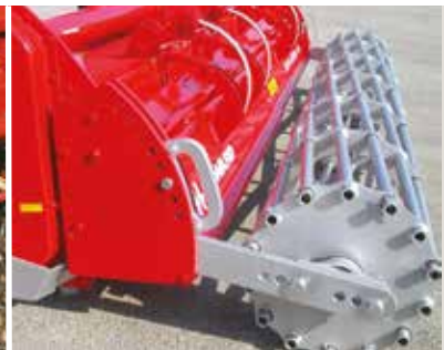
Compact depth control system for rear wheels and rollers.
