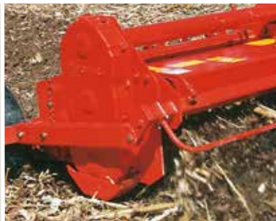
Rotavator is the most effective system for crumbling and residues incorporation.
