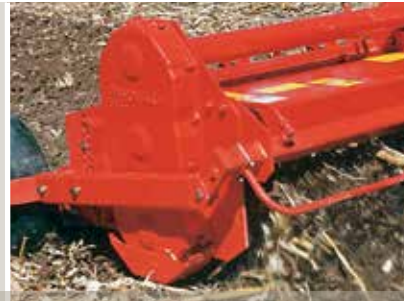
Rotavator is the most effective system for crumbling and residues incorporation.
