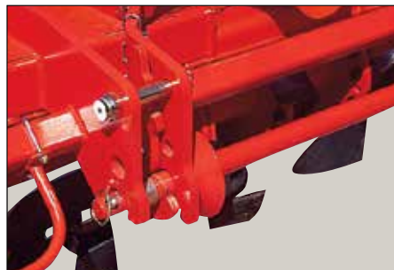
Linkage cat. 3 and 2 with quick coupling.
