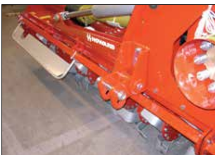
3 point linkage cat. 3 with floating lower links.
