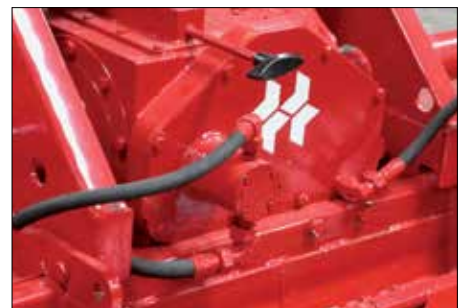
Rotavator 700S-D gearbox. Lever change gearbox and oil cooling system.
