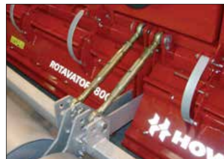
Detail of the combi hinged trailing board and depth control.
