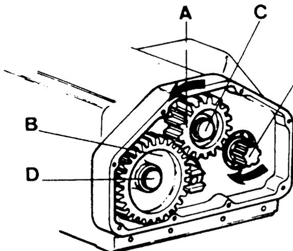
using the special gears A = 23 teeth and B = 27 teeth. The higher range of rotor speeds will be:
