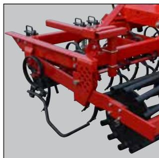
Depth adjustment with pin/hole system.
