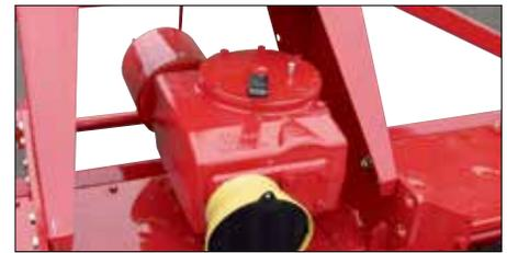
3-speed leverchange gearbox with rear PTO.
