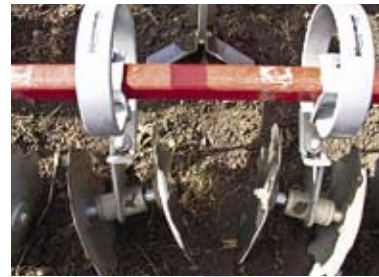
To help produce a more uniform finish, the levelling discs' original one-way position...
