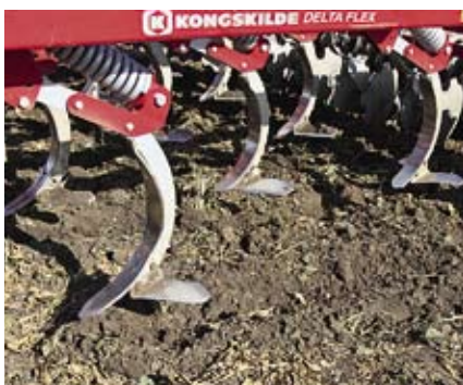
Uneven tine wear between front and rear is typical on a three-row design, but this can be reduced by ensuring the cultivator runs level. Kongskilde plans to shrink the tine wing width by around 12mm per side on production cultivators.
