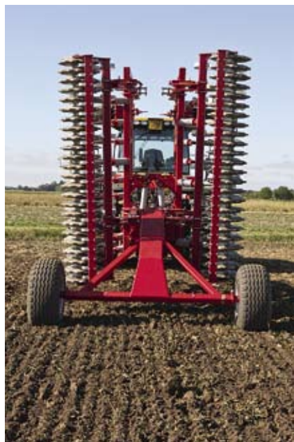
Folding up to 2.80m, the widest part of the trailed 6m Delta Flex model in transport is its wheels.
