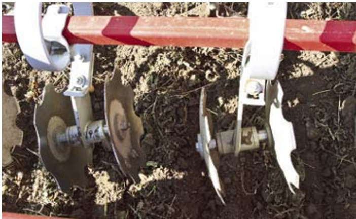
To help produce a more uniform finish, the levelling discs' original one-way position...
